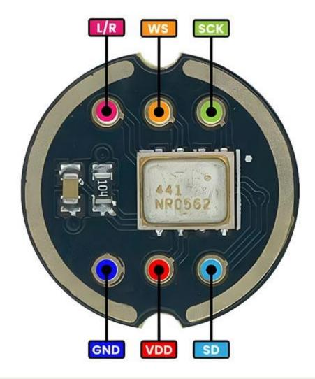
INMP441 Microphone INMP441 Microphone Pinout
